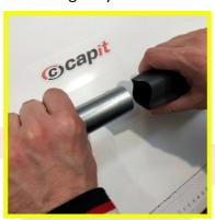
Stop the sleeve 50mm from the tube end.
